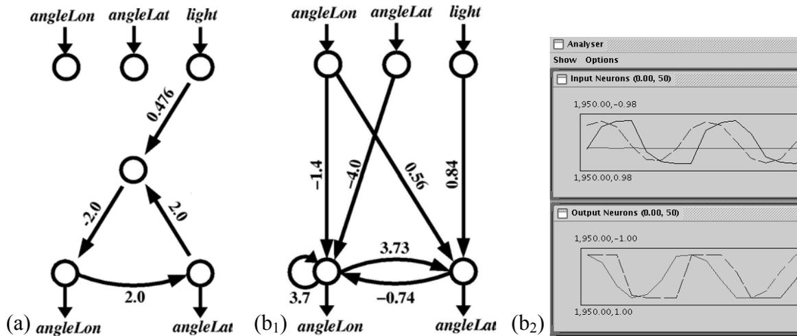
**Fig.7 Evolved networks for the centre motors of the salamander (phototropic task): a simple oscillator module (a) with the proper phase shift to move forward and a more advanced one (b<sub>1</sub>) with a smoother, more adaptive walking pattern (b<sub>2</sub>).**
