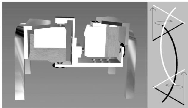
**Fig.4 The simplest realisation of the bending principle.**
