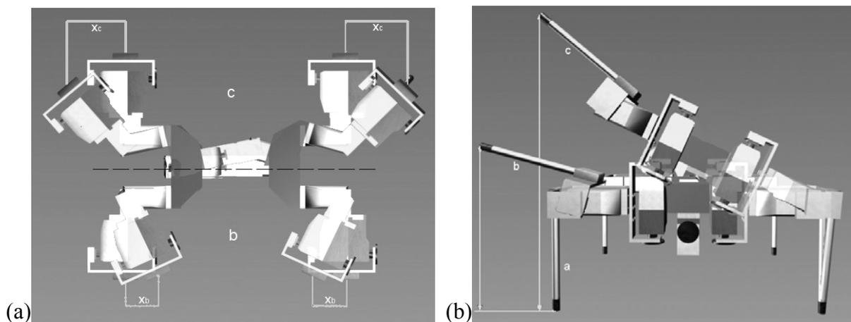
**Fig.6 The range enhancements of lateral bending (a) and longitudinal rotation (b)**
