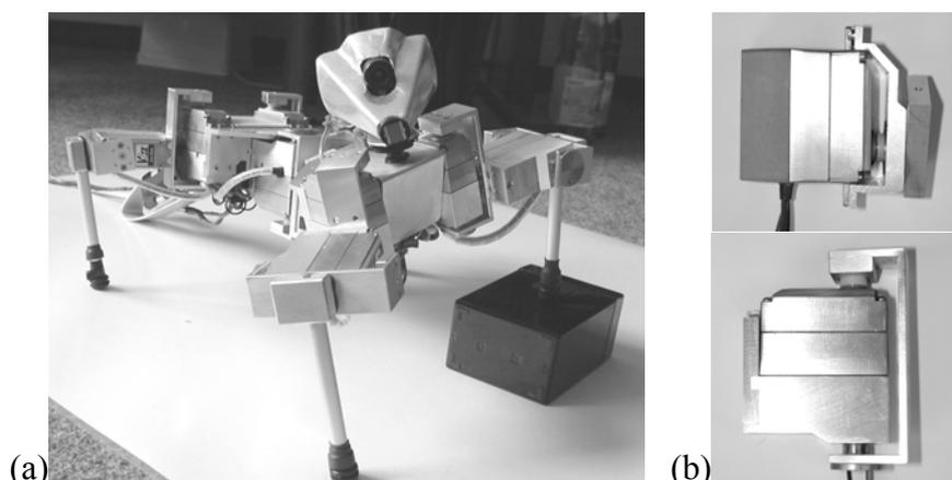
**Fig.5 The first prototype of the Robo-Salamander robot (a), constructed with the joint-modules of the AIS-Walking-Robot-Kit (b)**
