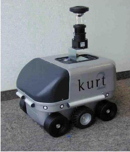
Figure 1. Robot *kurt-2* equipped with omnidirectional camera on top.
